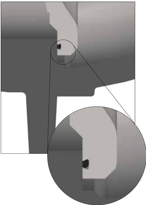
The TOM WHEATLEY swing check valve features a seat that is integral with the standard body. As an option, a renewable seat is field serviceable and facilitates the use of corrosion-resistant steels, overlays, and seat styles. Renewable seats are securely mounted inside the valve body using fasteners.
