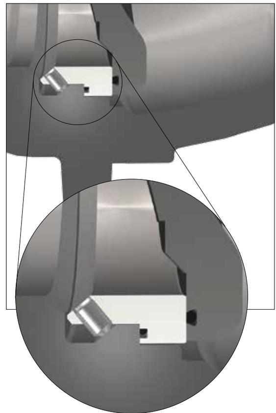
The renewable seat option allows the repair or replacement of all the seat sealing elements in the valve. By having both the seat and clapper as separate parts from the body, a damaged valve can be restored to as-new condition and performance. A renewable seat also facilitates use of different corrosion-resistant materials and modified seat designs to accommodate pipeline pigs.
